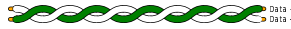
Figure 84: Twisted pair. The same signal is sent over both wires, but with opposing current polarity. Because the noise has the same polarity it can be filtered out by a differential amplifier. (Image: Wikipedia).
