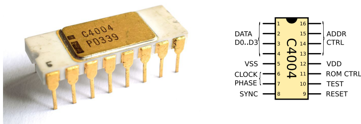
Figure 104: Left: DIL chip of an Intel 4004. (Wikipedia) Right: pin-out of chip.
