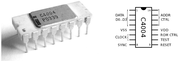
Figure 97: Left: DIL chip of an Intel 4004. (Wikipedia) Right: pin-out of chip.
