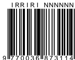
Fig. 5.45: Example of a barcode with the type of coding for each digit indicated above. Because the non-coded digit before the barcode is a 9, the first 6 coded digits are coded by 'IRRIRI' (I is inverse, R is reverse), see Tables 5.XI and 5.XII. The rest of the digits, after the synchronization pattern in the middle, are coded normally (N)
