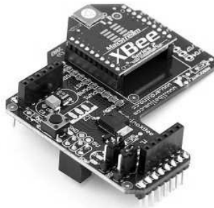
Fig. 5.53: XBee module on an Arduino XBee shield
