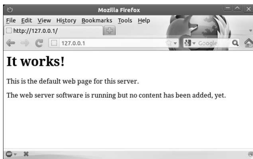
Fig. 5.58: Opening a browser on the server computer and point it to the home page of the computer itself ('local host' = http://127.0.0.1/ )
