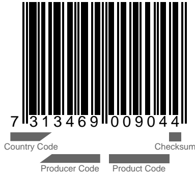
Fig. 5.46: Items of a barcode. The first two or three digits (including the non-coded digit) are the country code. The next digits, up to the half-way synchronization pattern are the producers code. The digits after the synchronization pattern are the product code
