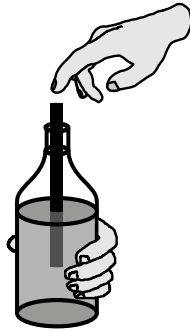
Fig. 3.8: Leidse Fles (Leyden jar), effectively a capacitor
