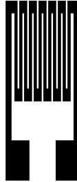
Fig. 4.22: Strain sensor (gauge). Changes in length are translated into changes in resistance
