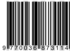
Fig. 5.44: Example of a barcode (of the Scientific American magazine). The individual digits of the code are highlighted by gray background for every odd digit (this is not part of the barcode, of course)
